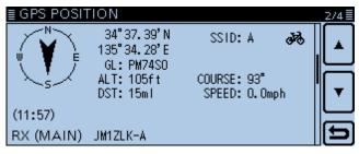
Example: When the caller's TX format is D-PRS Position (Mobile)
