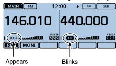
Transmission is automatically cancelled according to the "Hang Up Time" item setting.
