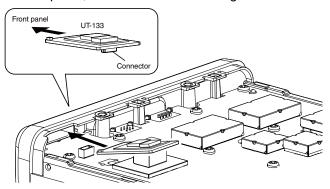
⚠ WARNING! BE SURE TO disconnect the DC power cable before starting the following procedures.
