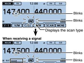
The S-meter shows the received signal strength.
