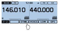
3 Touch the desired DTMF memory channel to transmit.
