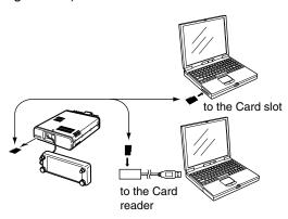
• Cloning from a PC using an optional cloning cable (see page 13-15)
