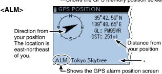
\*When a name is not assigned to the memory channel, date and time are displayed instead of the name.
