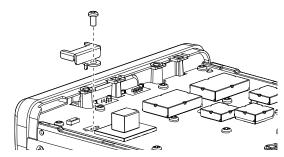
4 Place one end the UT-133 under the edge of the front panel, with the connector facing down.
